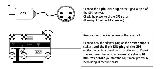
**Caution:** If the 5 pin DIN plug of the GPS an the power supply is connected on the motherboard, the WM Professional switch's automatically to the measuring mode *quartz*. This is the standard mode to adjust the time base by GPS.
