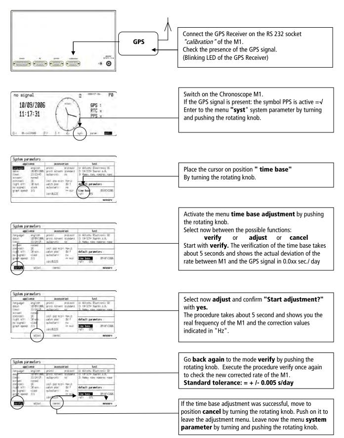
The instrument has to be **on-state** during **10 minutes before** you start the adjustment procedure.
