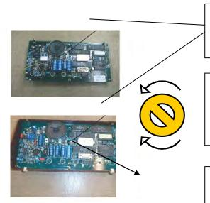
Select a screwdriver with blade size 2-3mm and place it carefully into the trimmer screw head / slit. (On the motherboard, there are two possible positions of the trimmer)
