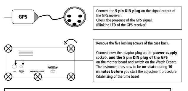
**Caution:** The time base adjustment by GPS on the Watch Expert's (red cases) is only possible for instruments **with a serial number**  $\geq$  **3000**. Starting from this serial number, the instruments are equipped with the additional measuring mode *quartz*. This automatically selected standard mode to adjust the time base by GPS.
